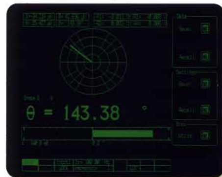
Figure 2 - Polar plots illustrate the signal as a vector relative to the reference signal.
